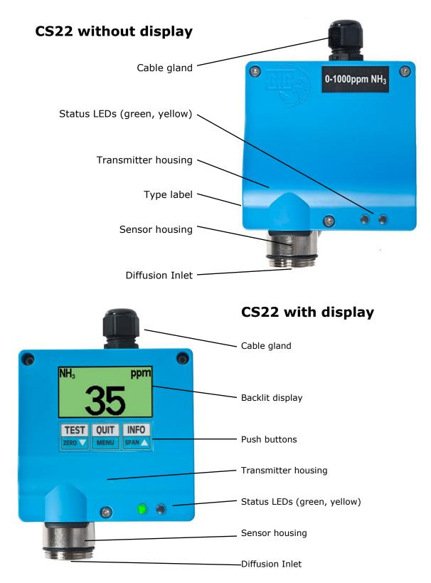
The transmitter housing contains the gas sensor and the transmitter electronics. The electronics converts the measuring signal into a gas concentration which is then signaled via an analog current signal of 4-20 mA or 0.2-1 mA or a digital RS-485 bus signal using the Modbus RTU protocol. In the display variant, gas concentration and status information are displayed.
