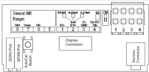
If the button is already released during the 1st phase, i.e. too early, then no adjustment is made and the measuring operation is continued as normal.
